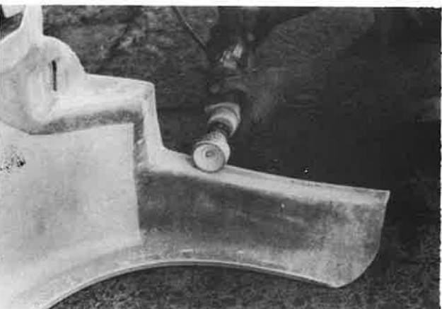
E127 Pay particular attention to flanges to avoid gaps or unevenness when bolted against the other panels.
