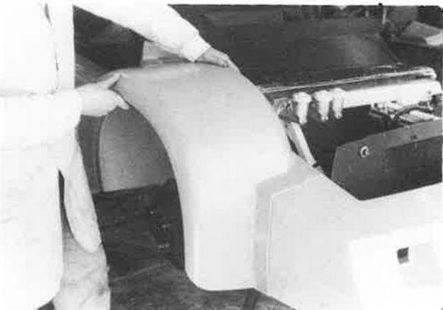
E126 Trial fit the front mudguard mouldings and relieve where necessary. The guard-to-nose panel joint, inside the bonnet opening, may retain a gap between the two panels. This is of no consequence.
