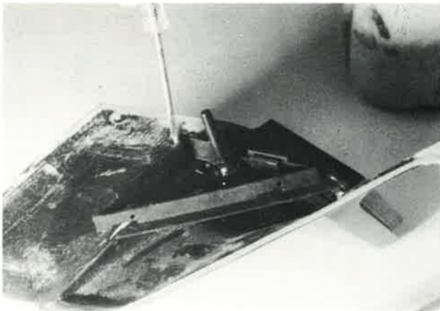
D 45 Secure mirror assembly in outer frame using a 3/16" Whitworth countersunk metal thread, 31mm. (1 1/4") long. Screw two self-tapping screws through the countersunk holes in the outer edge of the mirror housing and into the mirror assembly.
